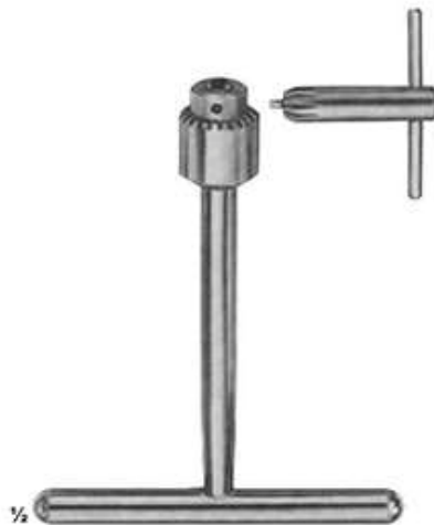
23-155 Drilling chuck, cannulated, for shanks up to 4.5 mm diam., And for triangular shaft width across flats 4.7 mm
